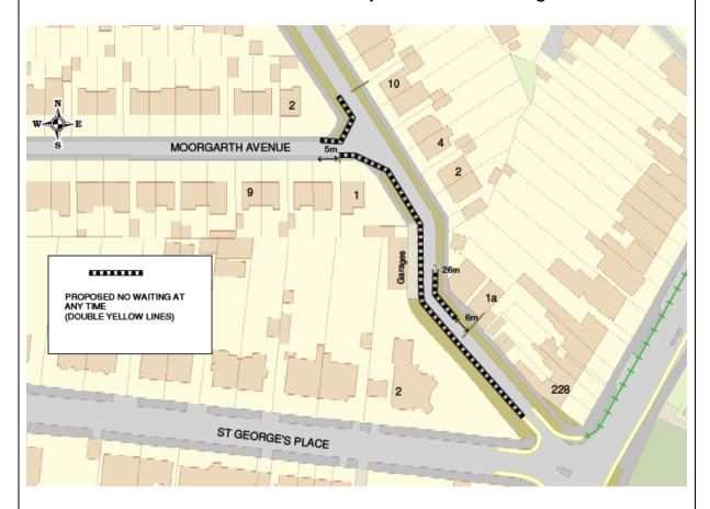
The proposal was designed to protect the bend and prevent displaced parking moving to the other side of the carriageway between St George's Place and Moorgarth Avenue.
